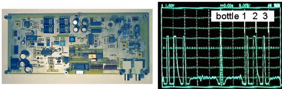
**Figure 14:** Professor Joe Paradiso's optimized tag reader board (left), and an oscilloscope showing three spikes corresponding to the resonant frequencies of three different bottles (right).
