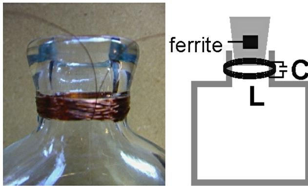
**Figure 13:** An electromagnetic resonator tag is wrapped around the neck of each bottle.
