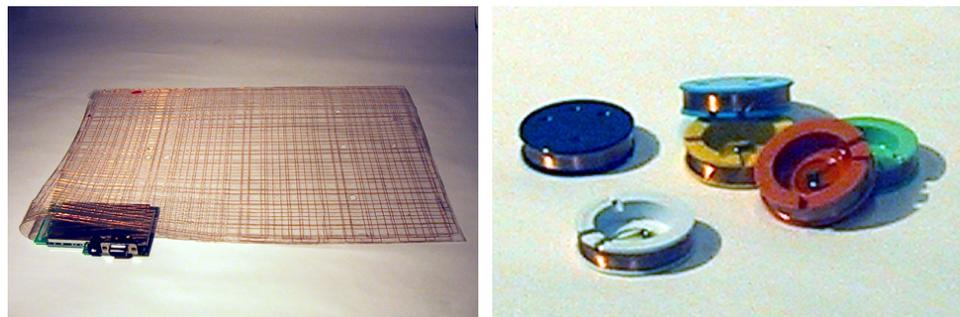
**Figure 36:** The tag-reading surface consists of eight antenna loops arranged in a flat plastic cover (left). The tags consist of a wire wrapped around the outside of a small plastic holder, in parallel with a capacitor concealed inside the holder (right).
